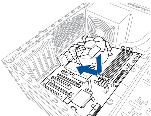
3. Place eight (8) screws into the holes indicated by circles to secure the motherboard to the chassis.
