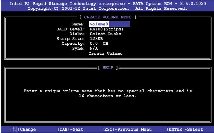
3. Press the up/down arrow keys to select a RAID Level that you wish to create then press <Enter>.
