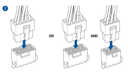
DO NOT connect the 6-pin power plug only, the motherboard may overheat under heavy usage.
