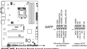
P10S WS Analog front panel connector
