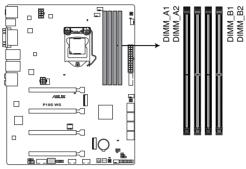
P10S WS 288-pin DDR4 DIMM socket
