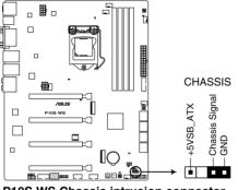
P10S WS Chassis intrusion connector
