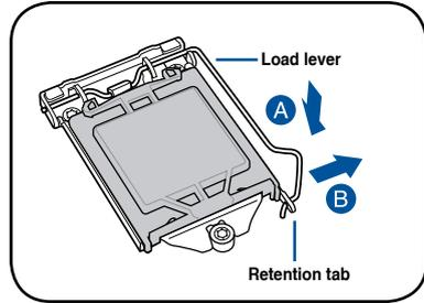
3. Lift the load lever until the load plate is completely lifted.
