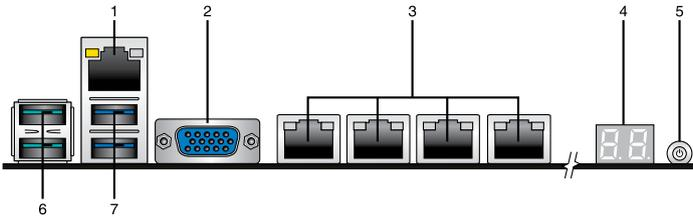
1. **RJ-45 port for iKVM:** This RJ-45 port functions only when you install ASMB9 management card.
