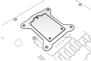
2. Use a Phillips screwdriver to tighten the four heatsink screws using the recommended sequence below.
