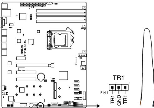
**P11C-E 4L Thermal sensor cable connector**
