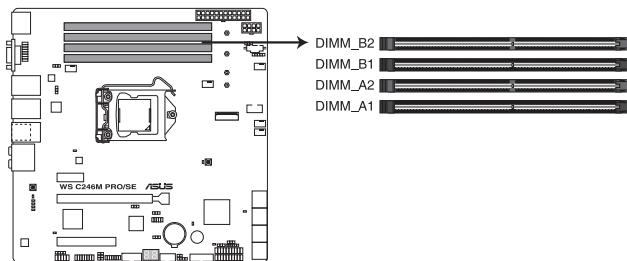
WS C246M PRO/SE 288-pin DDR4 DIMM sockets
