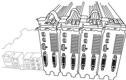
5. Connect four independent auxiliary power sources from the power supply to the four graphics cards separately.
