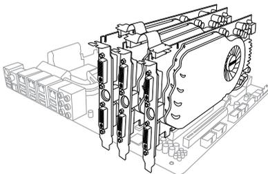
5. Connect three independent auxiliary power sources from the power supply to the three graphics cards separately.
