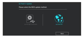
Press the Left/Right arrow keys to select an Internet connection method, and then press <Enter>.
