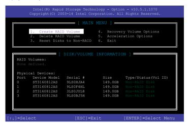
The navigation keys at the bottom of the screen allow you to move through the menus and select the menu options.
