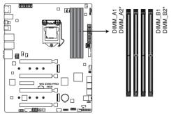
WS Z390 PRO 288-pin DDR4 DIMM socket
