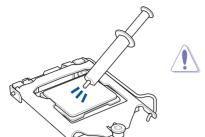
Apply Thermal Interface Material to the CPU cooling system and CPU before you install the cooling system, if necessary.
