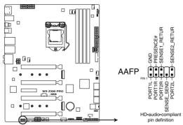
WS Z390 PRO Analog front panel connector
