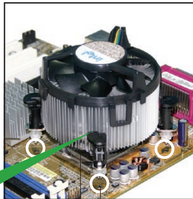
Motherboard hole Fastener
