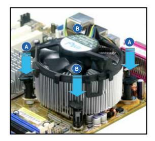
3. When the fan and heatsink assembly is in place, connect the CPU fan cable to the connector on the motherboard labeled CPU\_FAN.
