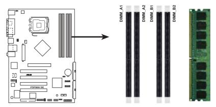
P5P800 SE 184-pin DDR DIMM sockets
