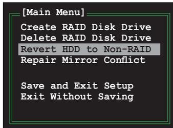
2. Use the space bar to select the HDD that you want to reset to non-RAID. A selected HDD shows a ► sign before it.
