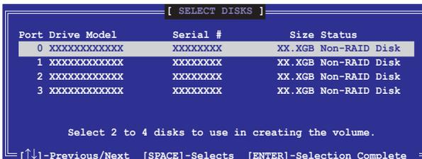
5. Use the up/down arrow key to highlight the drive you want to set, then press <Space> to select. A small triangle marks the selected drive. Press <Enter> after completing your selection.
