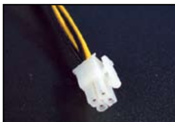
4-pin ATX connector
