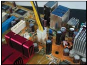
4-pin power connector (Konektor daya 4-pin)
