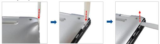
**IMPORTANT!** Avoid sliding the non-conductive pry tool along the side of your Notebook PC to prevent damage.
