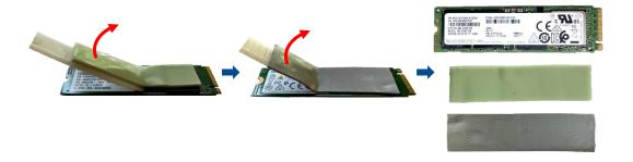
E. Paste the SSD D-PART PAD and the SSD PCB PAD to new M.2 card (SSD) front and back side.
