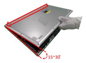
H. Put the base cover down slowly, and then press left and right side of base cover to fix, and press lower side of base cover to fix.
