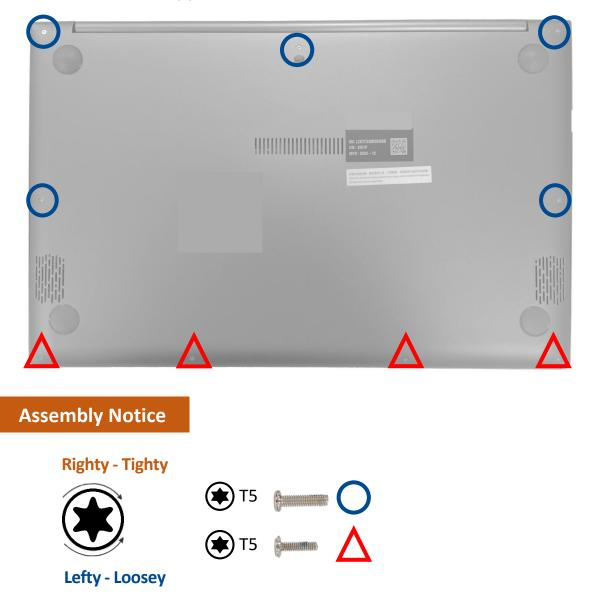
B. Use the non-conductive pry tool to lift open the indicated area of the base cover as shown in the illustration.
