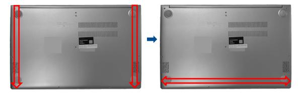
I. Secure the base cover in place using the screws.
