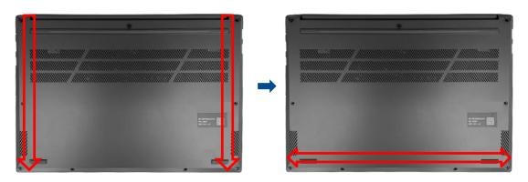
J. Secure the base cover in place using the screws.
