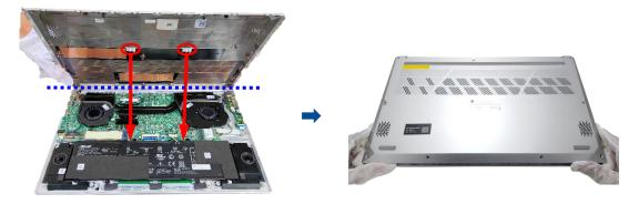
I. Please push down the base case follow direction of the arrow, then press down left and right side of base cover to fix, and press down lower side of base cover to fix.
