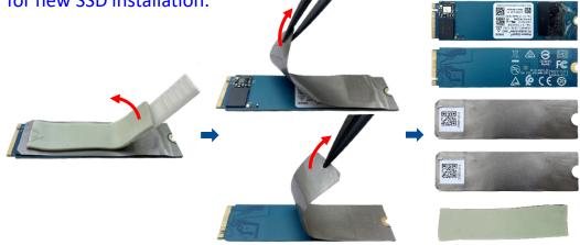
E. Paste the two ABSORBERS to new M.2 card (SSD) front and back side, then paste the THM SSD PAD\*1pc.
