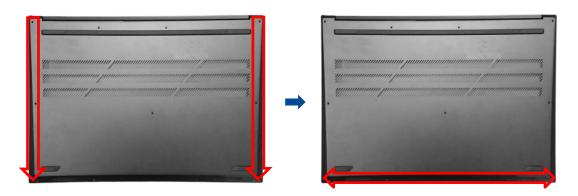
J. Secure the base cover in place using the screws.
