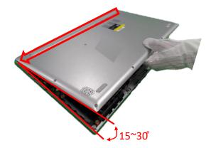
I. Put the base cover down slowly, and then press left and right side of base cover to fix, and press lower side of base cover to fix.
