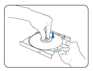
Slowly push the drive's tray back in. The drive will begin reading the table of contents (TOC) on the disc. When the drive stops, the disc is ready to be used.
