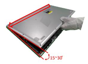
J. Put the base cover down slowly, and then press left and right side of base cover to fix, and press lower side of base cover to fix.
