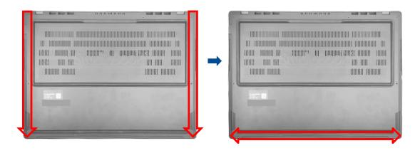
K. Secure the base cover in place using the screws.
