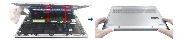
I. Please push down the base case follow direction of the arrow, then press down left and right side of base cover to fix, and press down lower side of base cover to fix.
