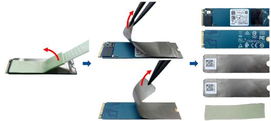
E. Paste the two ABSORBERS to the new M.2 card (SSD) front and back side, then paste the THERMAL PAD\*1pc.
