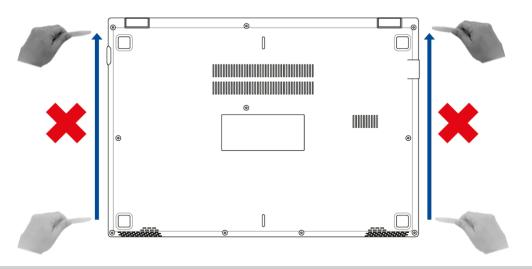
C. As illustrated, lift up the base cover slightly, and then push forward in the direction of the arrows, then lift up the base cover completely to remove it from your Notebook PC.
