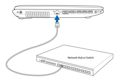
Network cable with RJ-45 connectors
