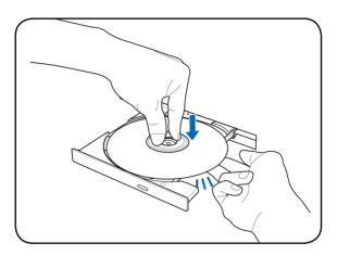
Slowly push the drive's tray back in. The drive will begin reading the table of contents (TOC) on the disc. When the drive stops, the disc is ready to be used.
