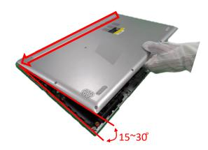
I. Put the base cover down slowly, and then press left and right side of base cover to fix, and press lower side of base cover to fix.
