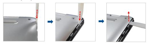
**IMPORTANT!** Avoid sliding the non-conductive pry tool along the side of your Notebook PC to prevent damage.
