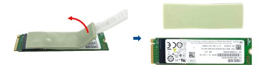
E. Paste the THERMAL PAD on the new M.2 card (SSD).
