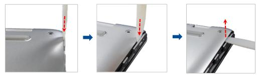
**IMPORTANT!** Avoid sliding the non-conductive pry tool along the side of your Notebook PC to prevent damage.
