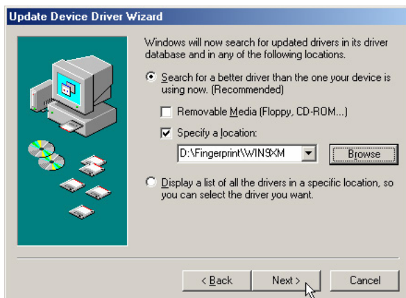
(5) Browse to the "Fingerprint" path for your operating system and click Next .
