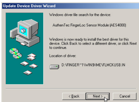
(6) Click Next when Windows finds the driver INF file on the support CD.
