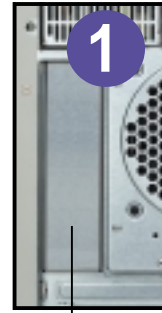
Temporary metal shield on the I/O slot opening
