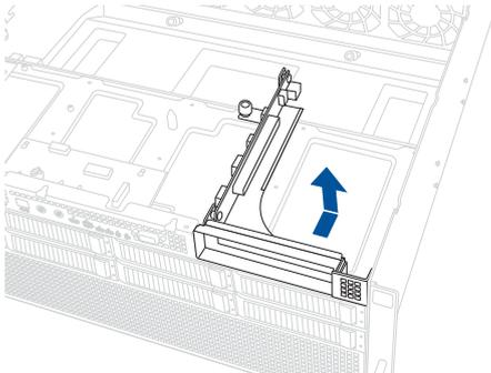
3. Push the metal bracket lock counter clockwise (A) until the metal bracket can be removed, then remove the metal bracket (B).
