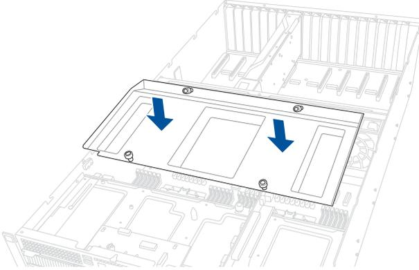
2. Tighten the four thumb screws to secure the air duct to the chassis.
