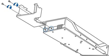
6. Align and insert the golden fingers of the GPU card into the PCIe slot on the PCIe SKU board, then secure it using the two screws removed earlier.
