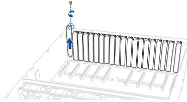
3. Align and insert the golden fingers of the PCIe card into the PCIe slot, then secure it using the screw removed earlier.
