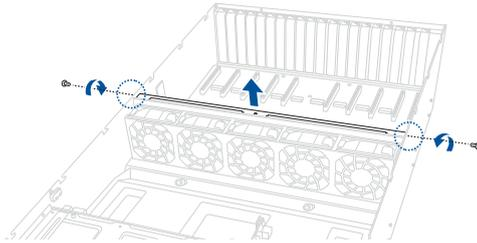
2. Remove the screws from the metal covers, then remove the metal covers.
