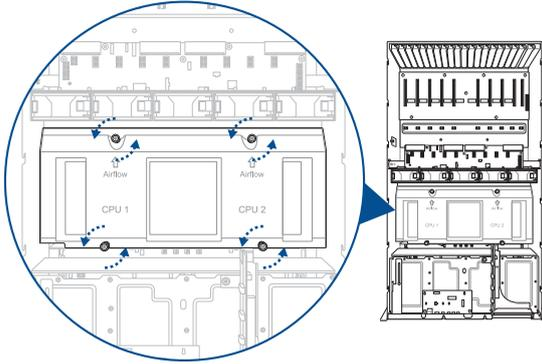
2. Lift the air duct to remove it from the motherboard.
