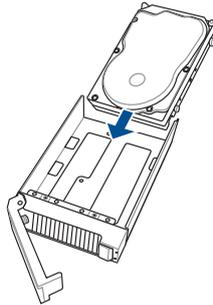
6. Carefully insert the tray and push it all the way into the storage device bay, then lock the tray lever to secure the drive bay in place.
