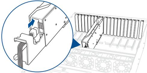
8. (Optional) For passively-cooled GPUs, install the additional air duct attachment.
