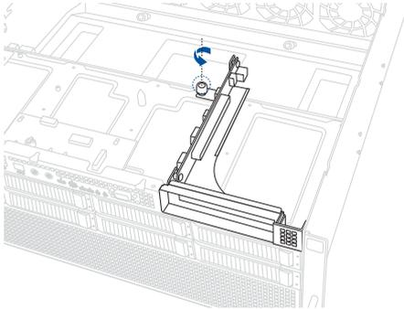
2. Firmly hold the riser card bracket, slide it towards the back of the chassis to unlock it, then pull it up to detach it from the chassis.
