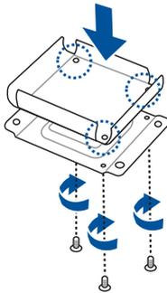
3. Align the screw holes on the Cache Vault bracket with the screw holes on the chassis, then secure the Cache Vault bracket with the two screws removed earlier.
