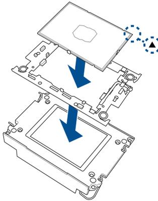
6. Align the CPU and heatsink assembly in the correct orientation so that the triangle marks on both the CPU and socket are aligned in the same direction, then place the heatsinks on top of the CPU sockets.
