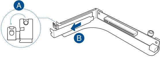
4. Insert the expansion card into the PCIe slot (A). Ensure that the golden fingers are totally inserted into the slot, then push the metal bracket lock clockwise until it locks and secures the expansion card to the riser card bracket (B).
