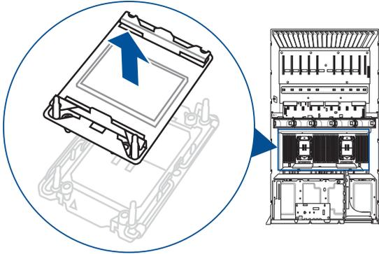
5. Attach the CPU to the carrier bracket, ensure the triangle mark is on the same side as the bracket lever, then attach the CPU and carrier bracket to the heatsink.
