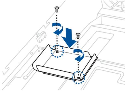
4. Align and install the Cache Vault Power Module into the Cache Vault Power Module clip.
