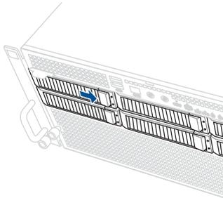
2. Firmly hold the tray lever and pull the storage device out of the bay.
