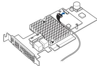
3. Follow steps 1-4 from the **Installing an expansion card to the front PCIe expansion card bracket** section to install the card to the riser bracket.
