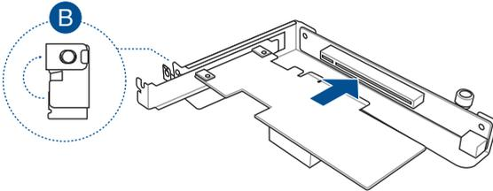
5. Align and insert the riser card and expansion card assembly into the chassis, then slide it towards the front of the chassis (A). Once in place, tighten the riser thumbscrew (B).
