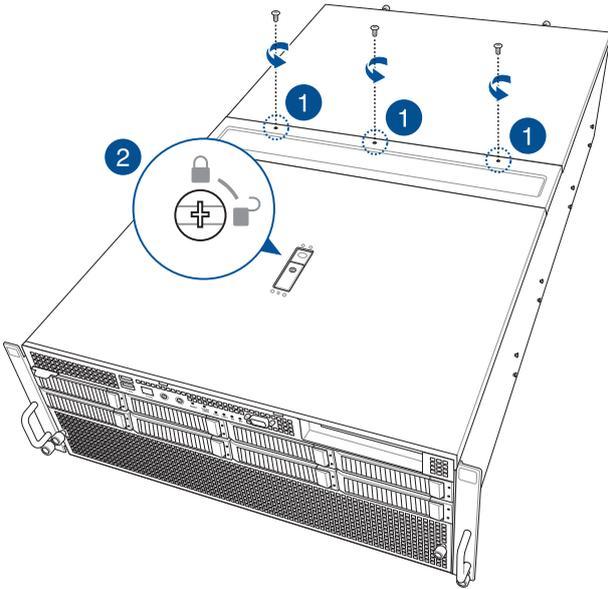
3. Press the spring lock to release the latch, then pull the latch upwards to disengage the chassis cover from the chassis.
