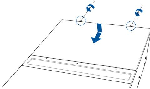
2. Secure the chassis cover using the three screws removed earlier.
