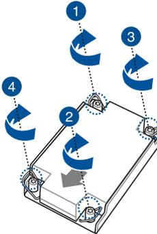
9. Reinstall the air duct. For more information, see the **Installing the air duct** section.
