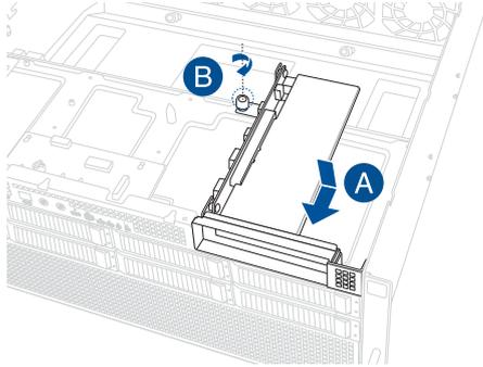
6. (Optional) Refer to the **Installing the Cache Vault Power Module** section to install and connect the Cache Vault Power Module.
