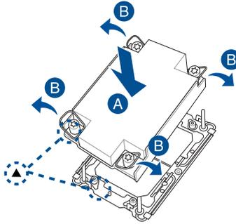
8. Do two (2) clockwise turns on each of the heatsink screws in the cross order pattern shown below until the heatsink screws are tightened and the heatsink is secured onto the motherboard.
