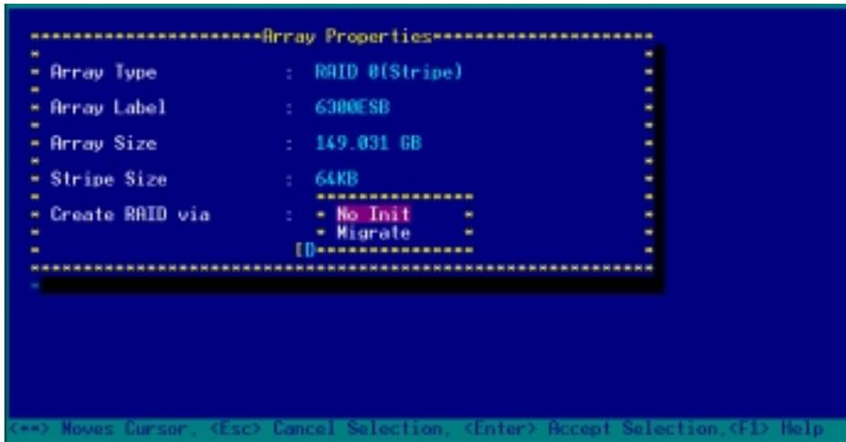
10. When you have finished setting the array properties, move the cursor to **Done**, then press <Enter> to create the RAID 0 set.
