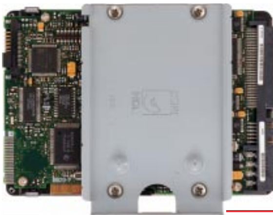
Hard disk drive mounted on carrier plate
