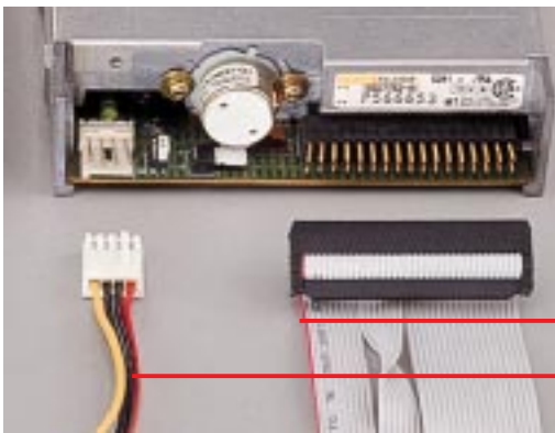
1.44MB floppy disk drive connections
