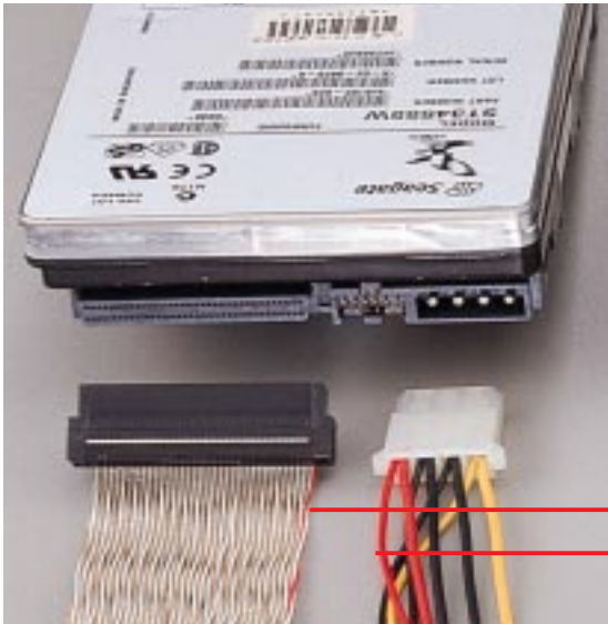
Ultra2 SCSI hard disk drive connections
