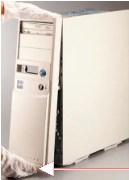
Removing the front panel
