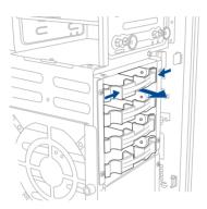
Carefully push the storage device tray lock pin out of the tray using a suitable tool.
