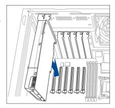
7. Secure the expansion card with the screw(s) that you removed earlier in step 4.
