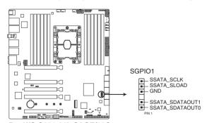
Pro WS C621-64L SAGE/10G Serial General Purpose Input/Output connector
