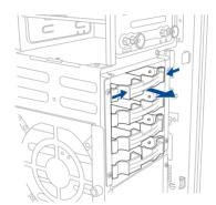
4. Align and insert the 3.5-inch storage device into the storage device tray ensuring that the screw holes on the storage device matches the HDD notches on the storage device bay. Ensure the storage device is seated firmly in the storage device bay.
