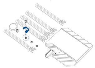
3. Align and insert the M.2 card into the M.2 slot, then secure it using a bundled screw.
