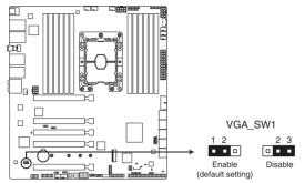
Pro WS C621-64L SAGE/10G VGA Controller jumper
