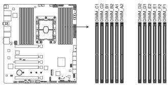
Pro WS C621-64L SAGE series 288-pin DDR4 DIMM socket
