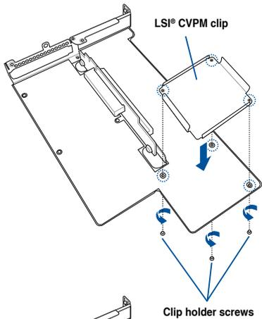
3. Install the CacheVault™ Power Module into the LSI® CVPM clip.
