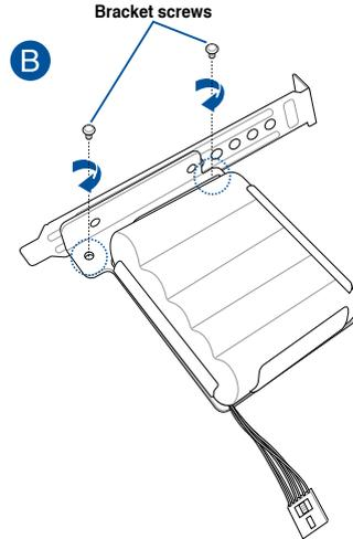
4. Install the CacheVault™ bracket assembly into a PCIe slot in your server system.
