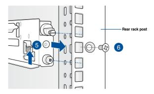
8. Lift the server chassis and insert it into the rack rail.
