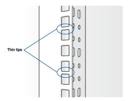
Press the spring lock, then insert the studs into the selected square mounting holes on the rack post.
