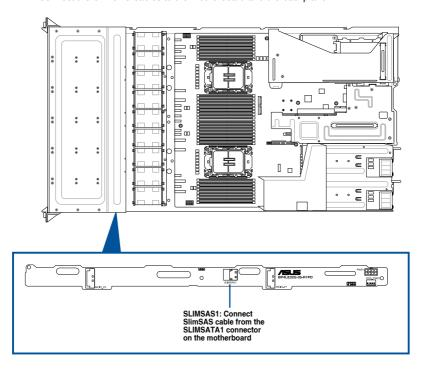
5. Tie the cables with cable tie(s) (A), then reinstall the backplane cover to the chassis (B).
