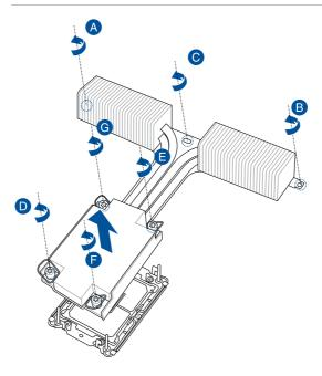
Flip the heatsink over to reveal the CPU and carrier bracket. Flip the carrier lever over to release the CPU, then remove the CPU from the heatsink and carrier assembly.
