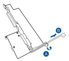
3. Install the expansion card to the **RS2\_PCIE1** slot on the butterfly riser card bracket (A), and then flip the metal bracket lock back to secure the card (B).
