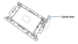
6. Remove the carrier bracket from the heatsink.
