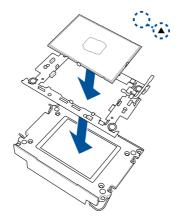
4. Remove the PNP cap from the CPU socket.
