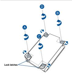
Completely loosen all the screws on the heatsink, then lift and remove it from the motherboard.
