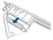
Place the 2.5" storage device into the storage device tray then secure it with four screws.
