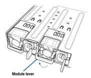
Hold the power supply module lever and press the PSU latch, then pull the power supply module out of the system chassis.
