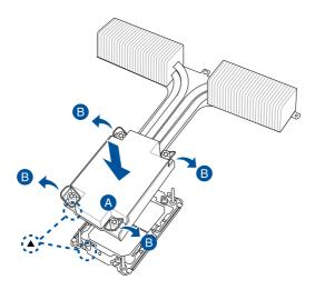
6. Do two (2) clockwise turns on each of the heatsink screws in the cross order pattern shown on the illustration until the heatsink screws are tightened.
