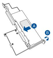
4. Align the butterfly riser card bracket to PCle slot B on the motherboard and push down until the butterfly riser card bracket is seated securely in the chassis.
