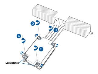
Completely loosen all the screws on the heatsink in the order shown, and then lift and remove it from the motherboard.
