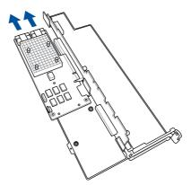
3. Remove the two (2) screws securing the card to the butterfly riser card bracket (A), and then remove the HBA/RAID card (B).
