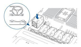
2. Connect the system fan cable to the fan connector on the motherboard.
