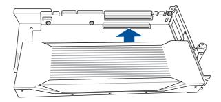
7. Once your expansion cards are installed, flip the metal bracket lock back to secure the expansion cards to the PCIe riser card bracket.
