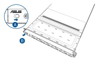
Slide the front bezel to the left to detach the front bezel, then remove it from the system.
