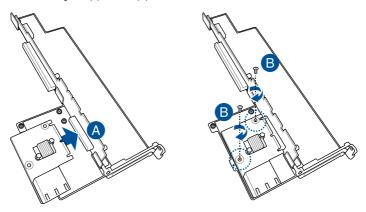
Follow step 4-5 of Installing an expansion card to the butterfly riser card bracket to install the butterfly riser card bracket to the chassis.
