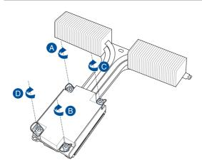
7. Tighten the remaining heatsink screws to secure the heatsink to the motherboard.
