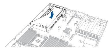
Replace the butterfly riser card bracket. For more information please refer to Installing an expansion card to the butterfly riser card bracket.
