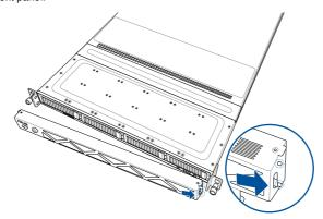
2. Push the bezel into the system until it clicks into place (A), and then slide the bezel release latch to the left to lock the bezel to the system (B).
