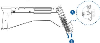
(optional) Install the GPU back bracket to the location shown in the illustration below using two (2) screws.
