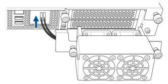
Connect the cables on the rear external fan to the REAR\_FAN1 and REAR\_FAN2
