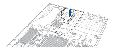
2. Flip the butterfly riser card bracket over, and then flip the metal bracket lock open (A) to remove the metal bracket (B).
