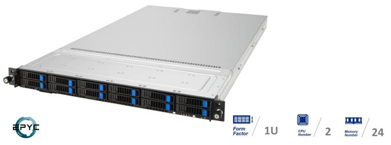
ASUS RS700A-E12-RS12U was designed to accelerate application performance leveraging accelerator cards and storage scalability. With the CPU and memory configured in a front parallel design that enables efficient airflow for excellent thermal performance, RS700A-E12-RS12U is optimized for rack placement.
