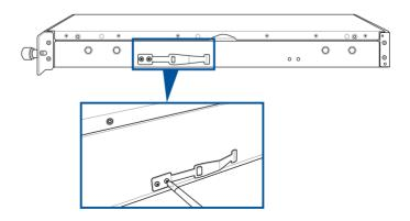
Select a desired space and place the appropriate rack rail (left and right) on opposite positions on the rack.
