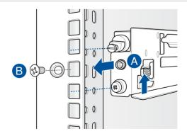
8. Lift the server chassis and insert into the rack rail.
