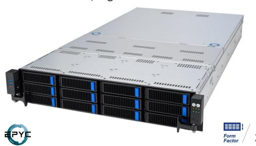
ASUS RS720A-E12-RS12 was designed to accelerate application performance leveraging accelerator cards and storage scalability. With the CPU and memory configured in a front parallel design that enables efficient airflow for excellent thermal performance, RS720A-E12-RS12 is optimized for rack placement.
