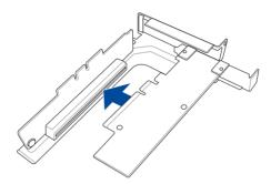
6. Align and insert the riser card and expansion card assembly into the PCIe slot on the motherboard.
