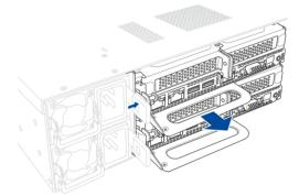
3. Firmly pull the server node out of the server chassis.
