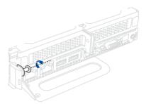
2. Hold the server node lever and press the green node latch.
