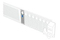
2. Firmly hold the tray lever and carefully pull the drive tray out of the bay.
