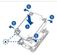
Do two (2) clockwise turns on each of the heatsink screws in the cross order pattern shown on the illustration until the heatsink screws are tightened and the heatsink is secured onto the motherboard.
