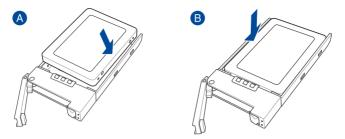
4. Align and insert the 2.5-inch storage device and drive tray assembly into the drive bay.
