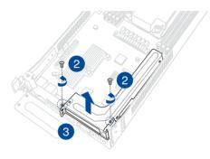
4. Remove the metal bracket from the riser card.
