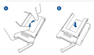
3. Follow step 4 of the **Installing a 2.5**" hot-swap SATA/SAS/NVMe storage device section to install the storage device and drive tray assembly into the drive bay.
