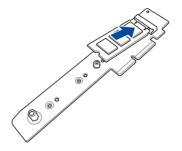
c. Push down on the M.2 card, then secure it to the M.2 baseboard using the screw removed previously.
