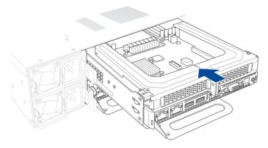
2. Secure the node latch using the screw previously removed.
