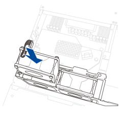
6. Connect the system fan cable to the fan connector on the midplane.
