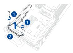
3. Remove the metal bracket from the riser card.
