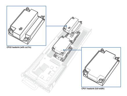
Once the heatsink is placed on top of the CPU socket (A), push the lock latches outwards on all four corners of the heatsink so that the heatsink and CPU assembly is secured to the CPU socket (B).
