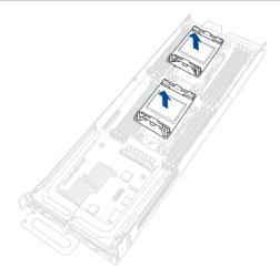
Align the CPU and liquid cooling module assembly in the correct orientation as shown in the illustration below, then place the liquid cooling modules on top of the CPU sockets.
