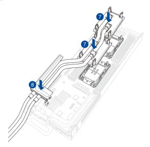
9. Once the liquid cooling modules are placed on top of the CPU sockets, push the lock latches outwards on all four corners of the liquid cooling modules so that the CPU and liquid cooling module assembly is secured to the CPU socket.
