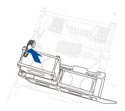
5. Insert the replacement fan into the fan compartment.
