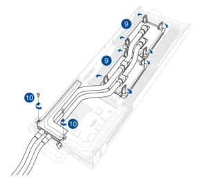
11. Do two (2) clockwise turns on each of the heatsink screws in the cross order pattern shown on the illustration until the heatsink screws are tightened and the heatsink is secured onto the motherboard.
