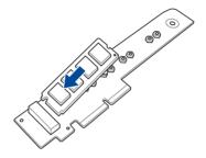
d. Push down on the M.2 card, then secure it to the M.2 baseboard using the screw removed previously.
