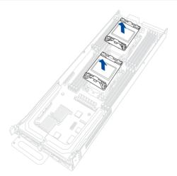
4. Attach the CPU to the carrier bracket, ensure the triangle mark is on the same side as the bracket lever, then attach the CPU and carrier bracket to the heatsink.
