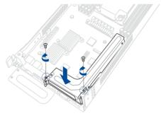
10. Refer to steps 6 to 7 in the previous section to reinstall the left riser card.
