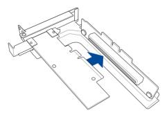
8. Align and insert the riser card and expansion card assembly into the PCIe slot on the motherboard.
