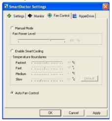
There are different fan speed levels (eg. medium, fast and fastest). The default value of the fan speed is medium. The fan speed automatically rises when GPU clock speed rises (see the figure on the next page), and also adjust to the fastest level while playing 3D games.
