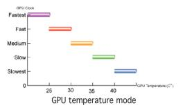
With the ASUS SmartCooling feature, the four temperature boundaries in the Fan Control page also defines the SmartDoctor thresholds for the GPU clock. In this mode, the lower the temperature, the better performance you can have.
