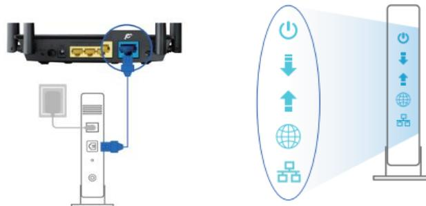
3. Plug in the power adapter and press the power button at the back of your router. Check the WAN and 2.4G / 5G LED lights to ensure the hardware connection is ready.
