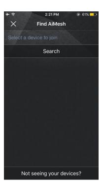
4. After click, it will search AiMesh node automatically. When AiMesh node shows on this page, click it to add it into AiMesh system. It is best to place all routers in close proximity when synchronizing for the first time in case of interference.
