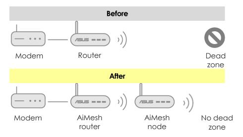
3. Put **AiMesh router** in the center of the house. We recommend various location placement examples.
