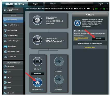
4. After click Search, it will search AiMesh node automatically. When AiMesh node shows on this page, click it to add it into AiMesh system. It is best to place all routers in close proximity when synchronizing for the first time in case of interference.
