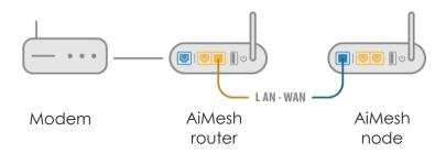
If you want to keep wired connection manually between AiMesh router and node, launch web GUI <a href="http://router.asus.com">http://router.asus.com</a>, and go to Network Map. Click on AiMesh icon, you will find the node list at the right side. And then click on the node picture → More Config → Connection Priority → Ethernet.
