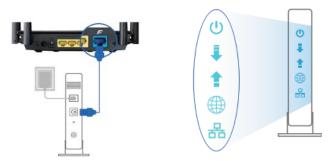
3. Plug in the power adapter and press the power button at the back of your router. Check the WAN and 2.4G / 5G LED lights to ensure the hardware connection is ready.
