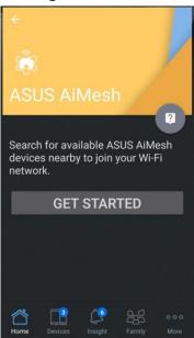
4. After click Get Started, it will search AiMesh node automatically. When AiMesh node shows on this page, click it to add it into AiMesh system. It is best to place all routers in close proximity when synchronizing for the first time in case of interference.
