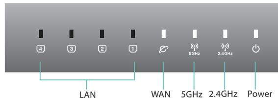
Check the WAN and 2.4G / 5G LED lights to ensure the hardware connection is ready (see the picture above).
