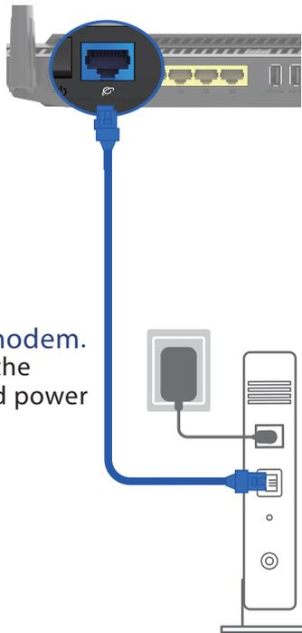
Power on the modem. Plug modem to the power outlet and power on.
