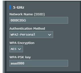
3. On the **Wireless name (SSID)** field, key in a unique name for your wireless network.
